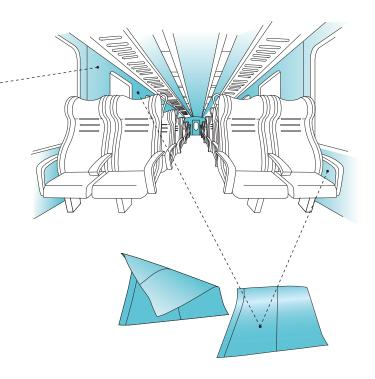
Thanks to their light weight and the many varied ways their material properties can be combined, composites are ideal for fitting out the interiors of passenger cabins, such as in the sides, window panels and luggage compartments. The areas shown in the illustration are just a few of many examples.
