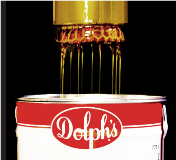
Dipping process for stator impregnation.
